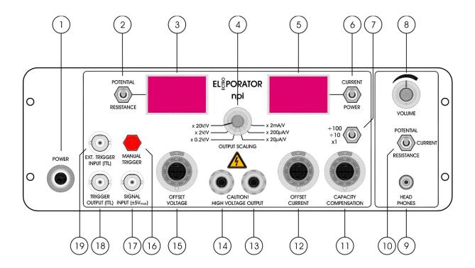
Figure 1: ELectroPORATOR front panel view
