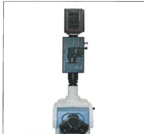
W-VIEW GEMINI and ORCA-Flash4.0 on an upright microscope
